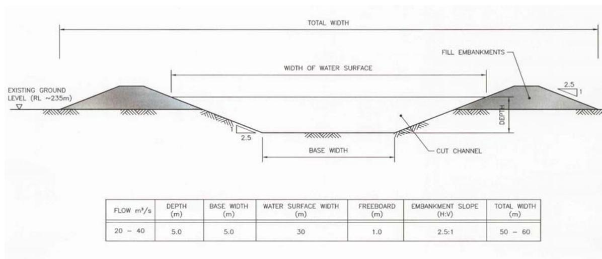
FIGURE 3-11: Cross section of the headrace
